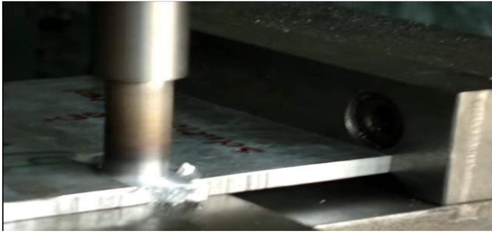
Figure 6.9: State of FSW welding after 25 seconds
