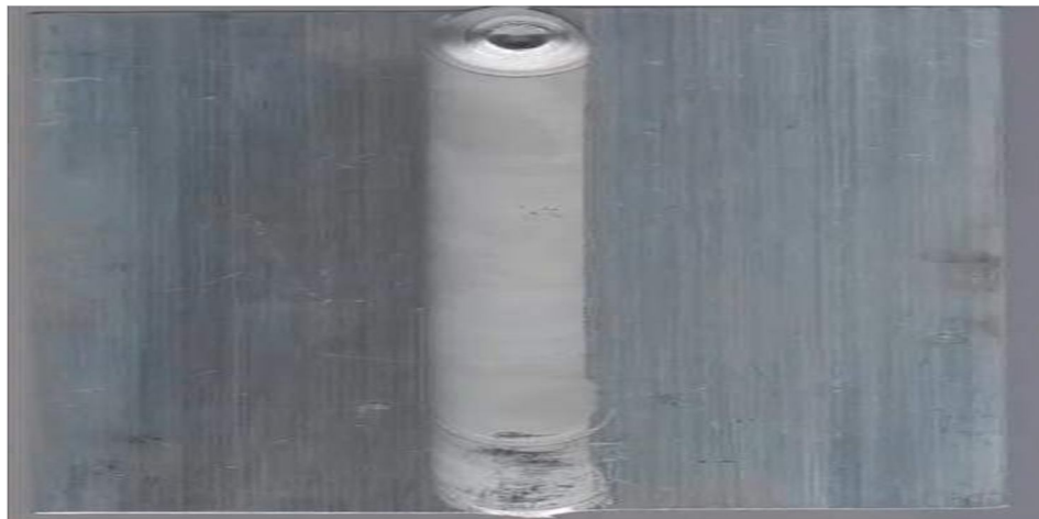
Figure 6.16: Final state of FSW welding
