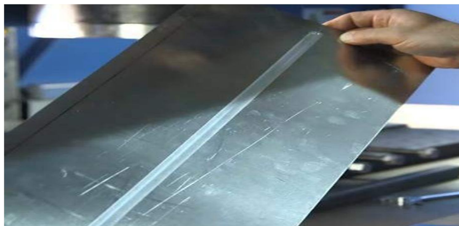
Figure 1.2: Displaying end product after applying FSW on plates of dissimilar aluminum alloys having series number AA6061 and AA6062
