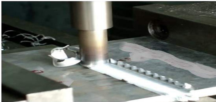
Figure 6.13: State of FSW welding after 205 seconds
