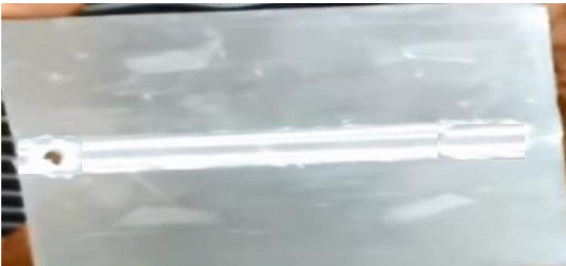
Figure 6.17: Final workpiece by performing FSW welding of AA2024 with AA6061
