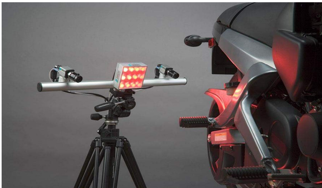
Figure 1.2: DIC is applied to find deformation, vibration and strain on material [38]
