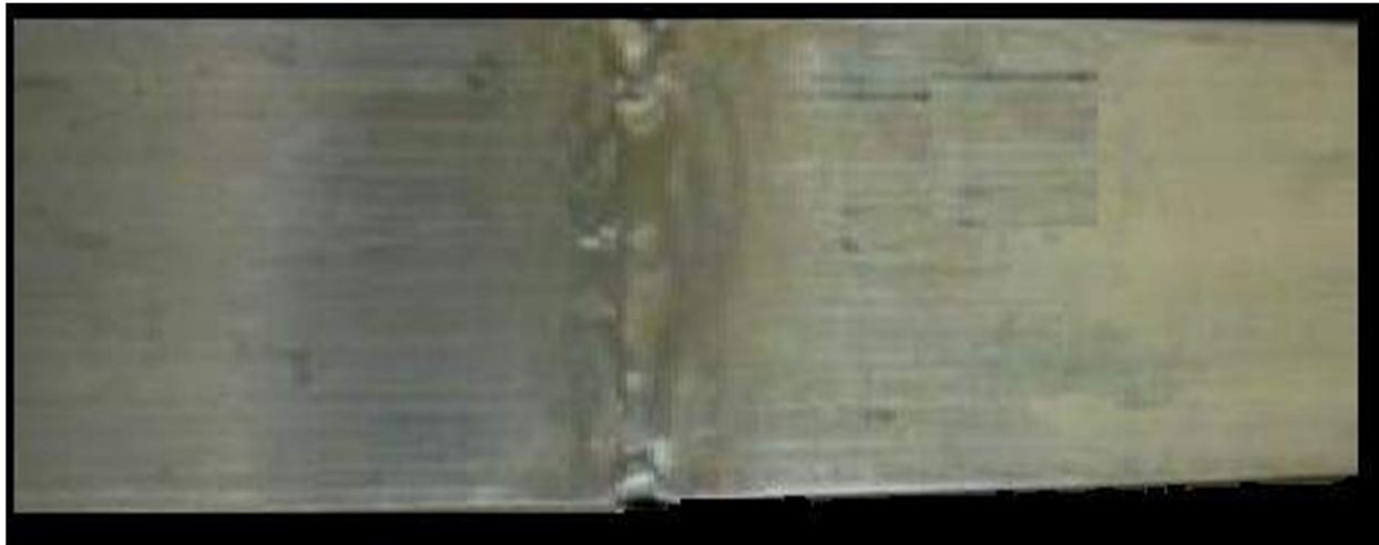
Figure 6.7: Friction stir welding product of AA6061-O and AA6061-T4 of second pair
