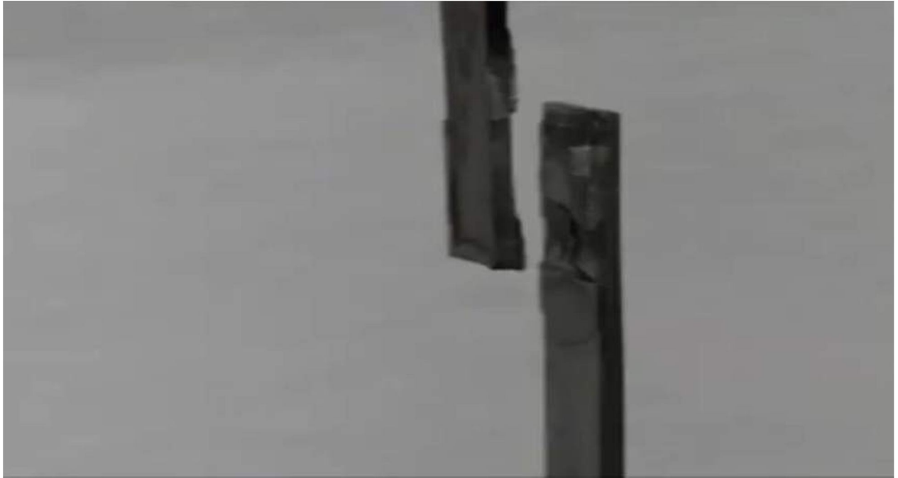
Figure 6.15: Failure of the single lap joint preparation after applying tensile stress Figure 6.15 is showing the final failure of the joint.
