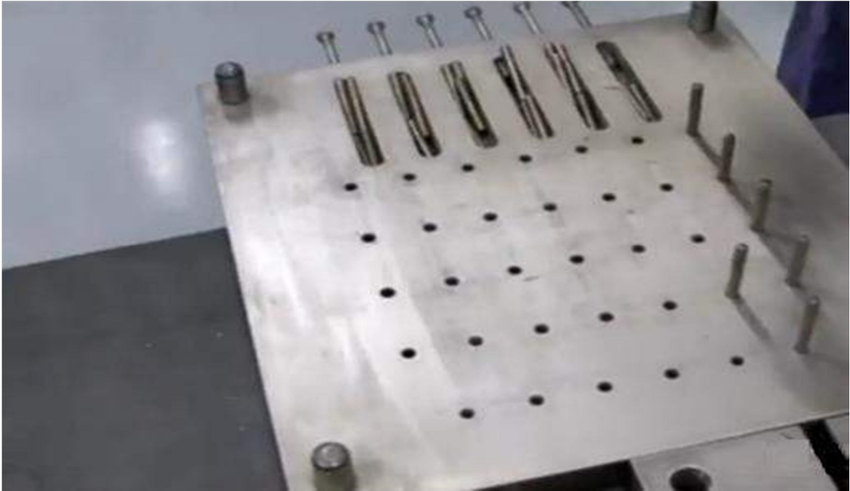
Figure 6.5: Single lap joint preparation setup
