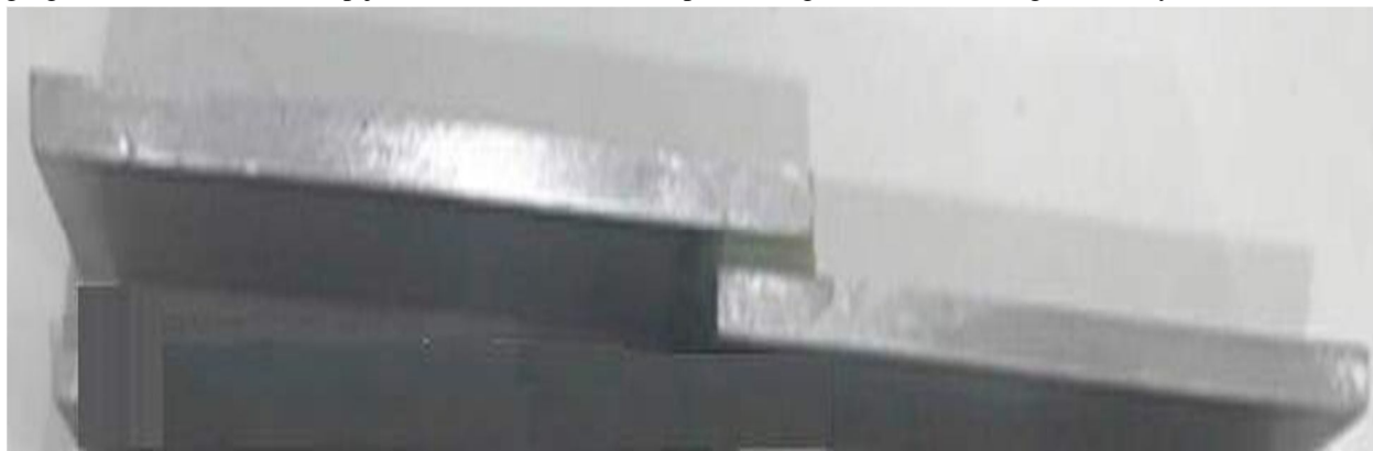
Figure 6.2: Lap joint number 1
