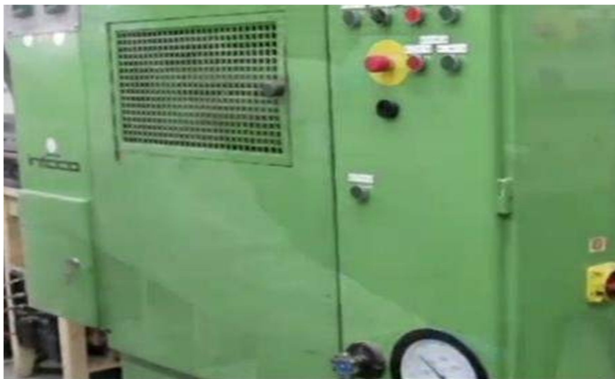
Figure 6.8: Heating machine for curing the single lap joint preparation
