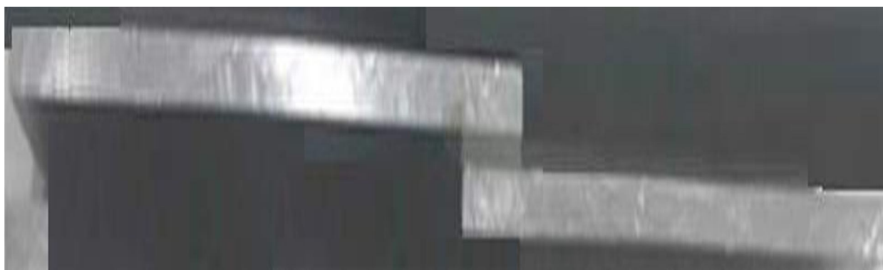
Figure 6.4: Lap joint number 3
