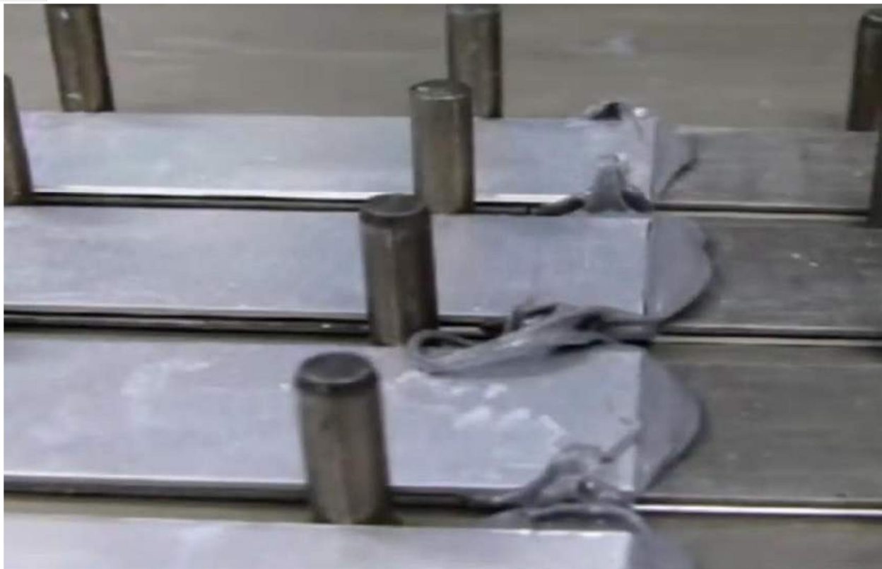
Figure 6.7: Adhesive is used for single lap joint preparation Figure 6.7 showing lap joints with the given adhesive.
