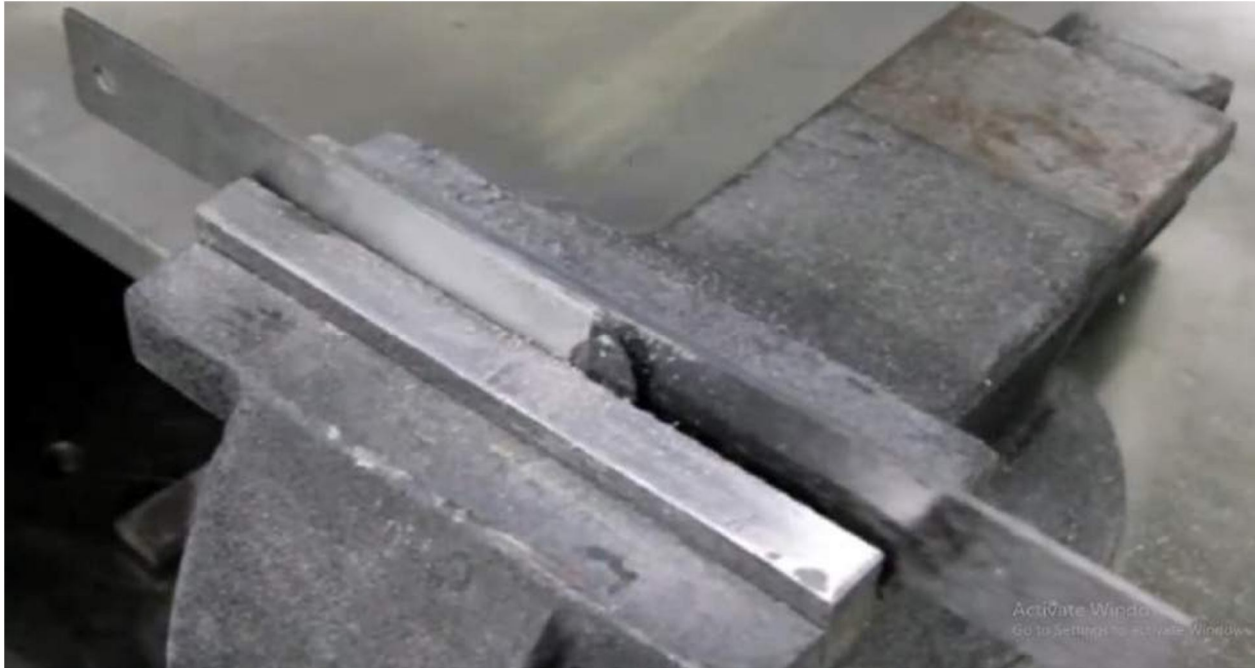
Figure 6.9: Removing unwanted material from single lap joint preparation
