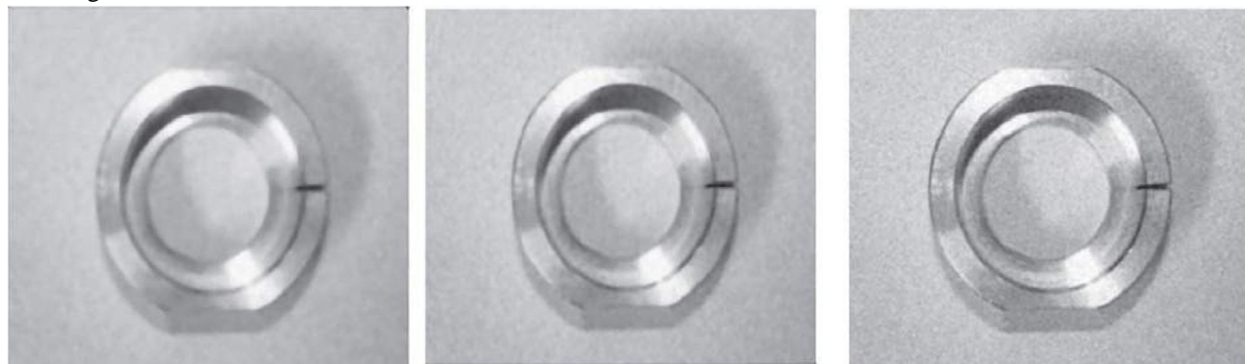
Figure 1.2: Median filtered image with different size windows of 3X3, 5X5 and 7X7.
