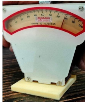
Fig. 7 Shore D hardness tester
