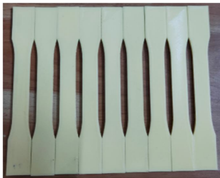
Fig. 3 3D printed specimen before testing
