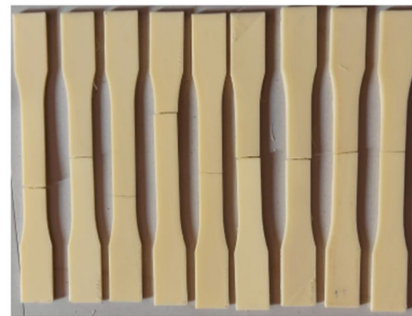
Fig. 4 3D printed specimen after testing
