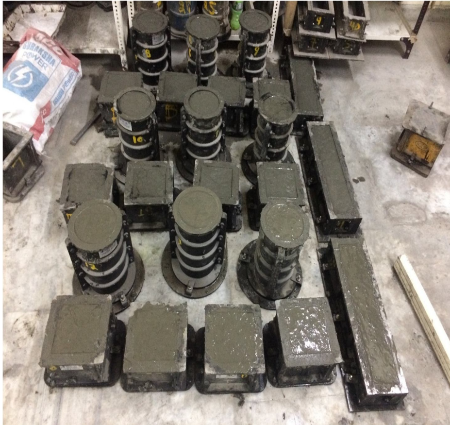
Figure– 1: Casted Samples for Hardened properties testing
