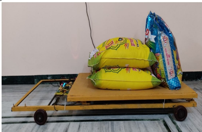
Fig. 14 Experimental setup under overload condition
