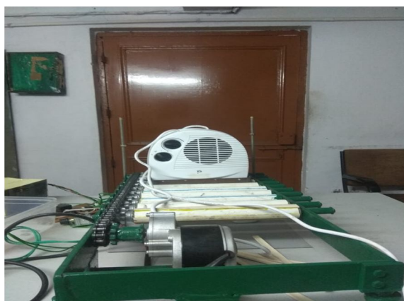
Fig-9: Figure showing final shrink wrapping for cloth peg with 250*250mm heater
