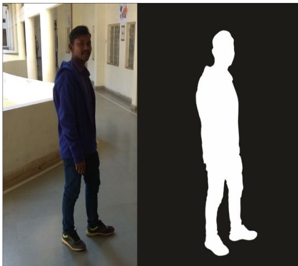
Fig. 7. Delta Image is put on entry threshold to obtain a motion black-white image
