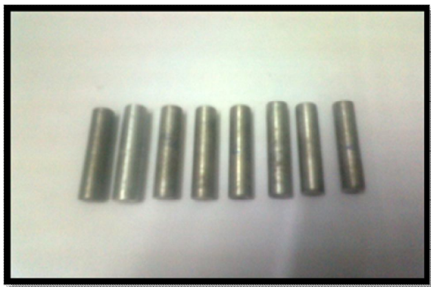
Figure: Sample for the wear testing
