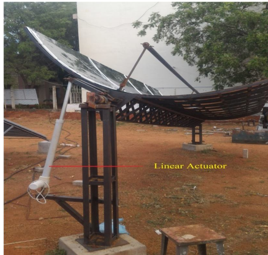
Fig 4 PTC assembly with Linear actuator
