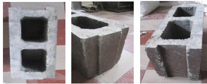
Interlocking ends of Designed Hollow Block
