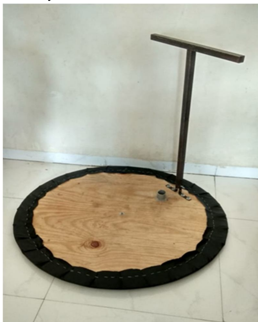
Fig 11. Air cushion material handling
