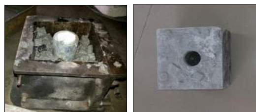
Cube Casted for Pullut Test
