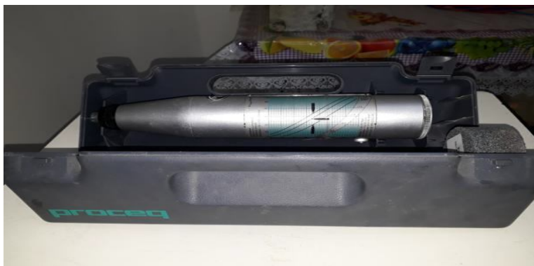
Fig. 2. Rebound Hammer Test
