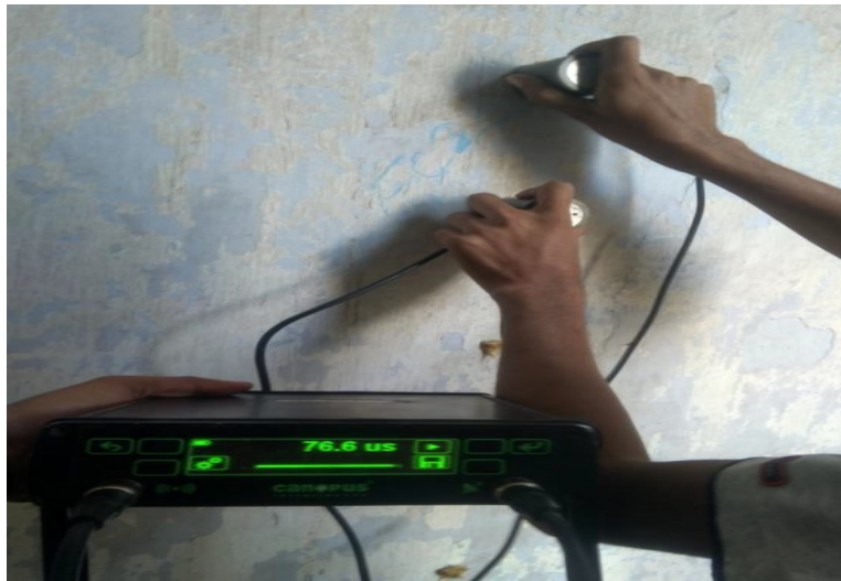
Fig. 1. Ultra-Sonic Pules Velocity Test
