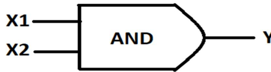
Fig.4. Basic AND Logic Gate
