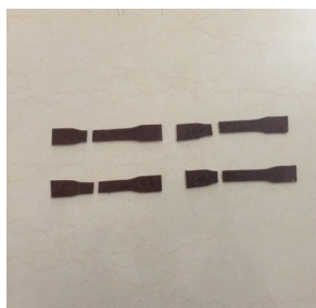
Fig 9 - Tensile test specimen after test
