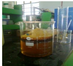
Fig 5: Alkaline treatment of natural fiber
