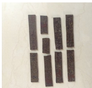
Fig 12 - Flexural test specimen after test
