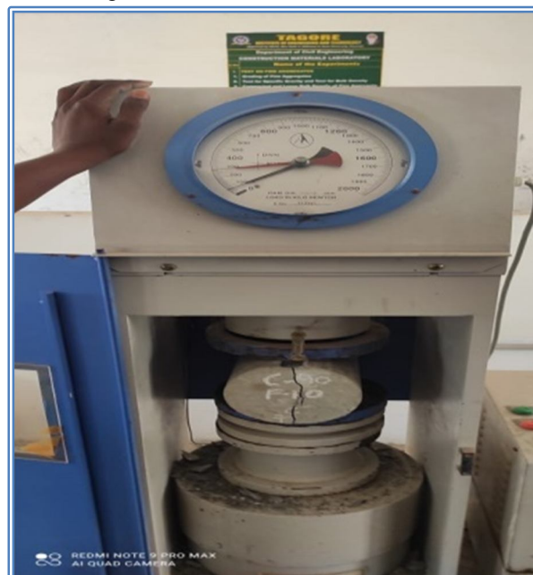
Fig.2. Split tensile strength test of cylinder specimen
