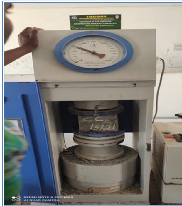
Fig.1. Compressive strength test of cube specimen
