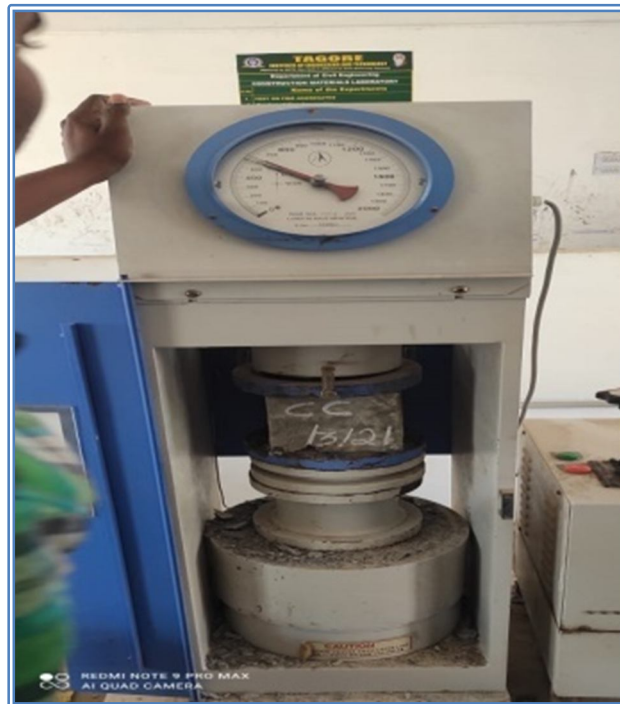
Fig.1. Compressive strength test of cube specimen
