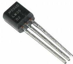
Fig. LM 35 Temp sensor
