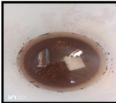
Sample 2 After Flocculation
