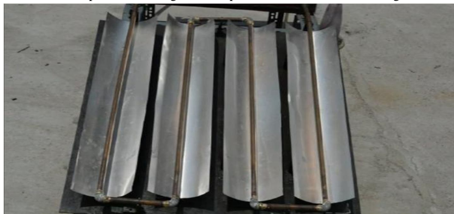
Fig 7. Thermosyphon Copper Loop with parabolic concentrator
