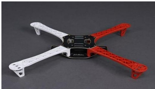
Fig.3 Drone Frame PA66GF30 Material
