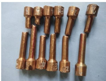
Fig. 1.11 Tensile Specimens after Test
