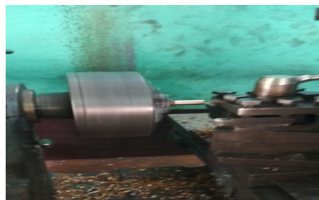
Figure:1.8 Machining of Casted Product
