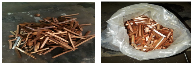
Figure1.2: Copper billets cut into small pieces
