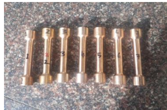
Figure 1.9 Tensile Test Specimens before test
