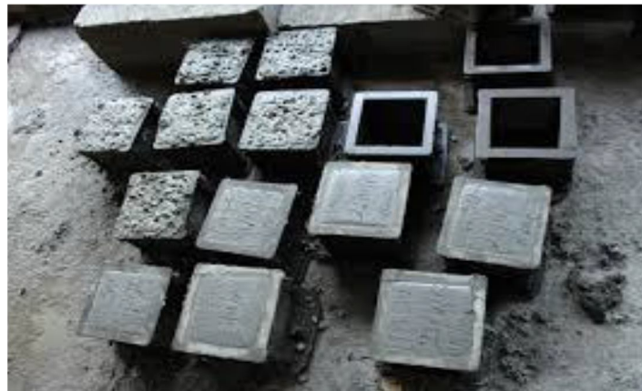
Fig2: Cube moulds prepared for the concrete
