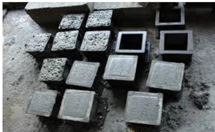
Fig2: Cube moulds prepared for the concrete
