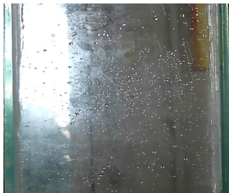
Fig. 3 Traditional TLD (consists of water as liquid)
