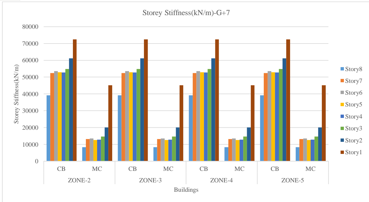
Fig.8: Storey Stiffness(kN/m) for G+7 building
