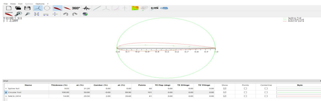
Fig -1: NACA 2414 Airfoil Design
