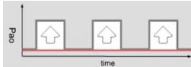
FIG 2.1 IPPV (intermittent positive pressure ventilation) [9]
