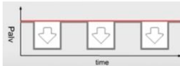
FIG 2.2 INPV (intermittent negative pressure ventilation) [9]
