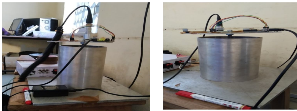
Fig.1 Actual setup along with FFT and Ardiuno accelerometer arrangement
