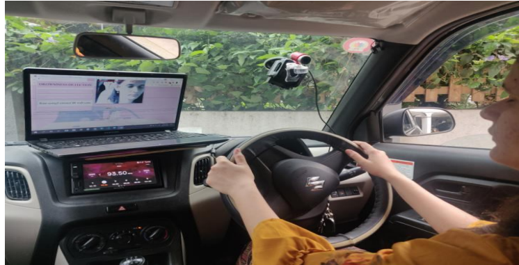
Fig 4.3: Drowsiness Detection using External Webcam.
