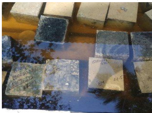
Figure 4: Curing of Geopolymer mortar cubes
