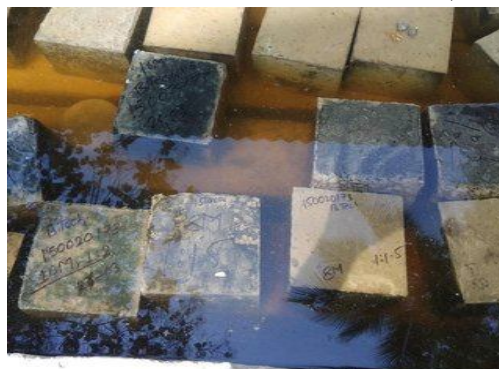
Figure 4: Curing of Geopolymer mortar cubes
