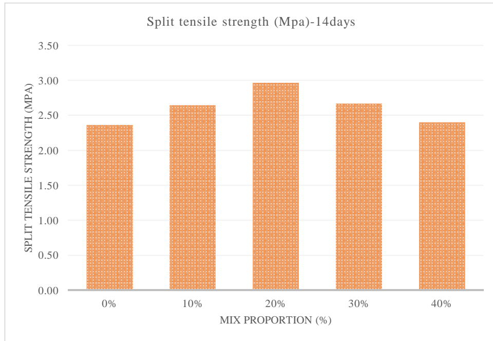
Figure 5: Split Tensile strength (14 days) of SCC with foundry sand
