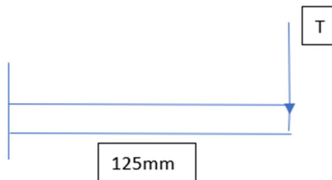
Figure No 2: Load on shaft
