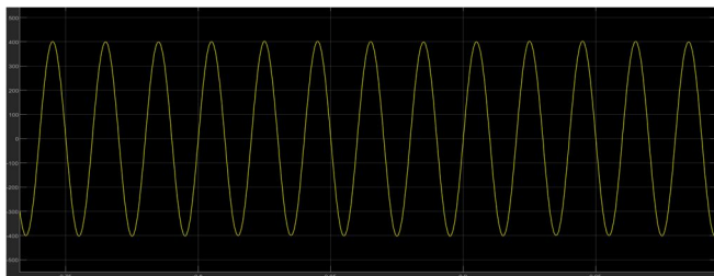
Fig .16 Output of Inverter after filtering
