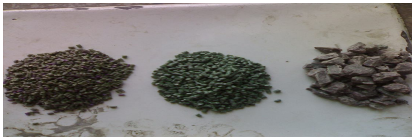
Figure.3.2. Three types of plastic aggregates (smaller, medium and coarser size)
