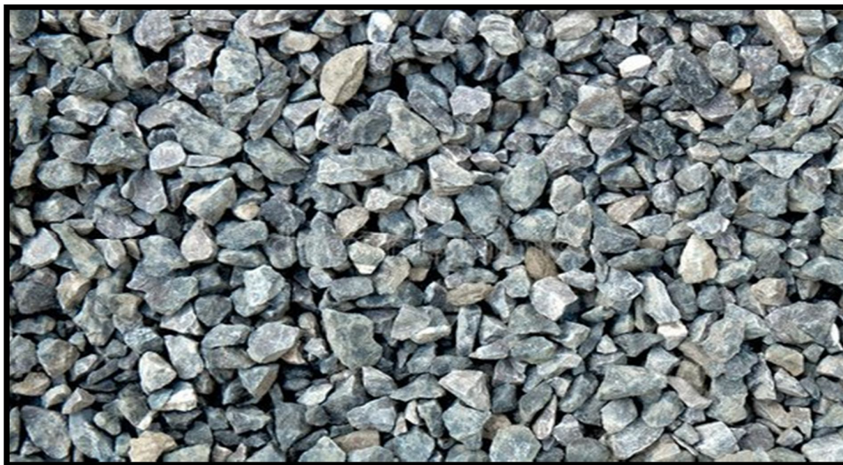
Recycled Concrete Aggregate
