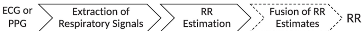
Fig. 1. Depicts the three steps of a respiratory rate (RR) algorithm that predicts RR from ECG or PPG data [43].
