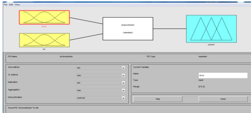
Fig. 4 FIS editor of fuzzy controller with 9 rule base
