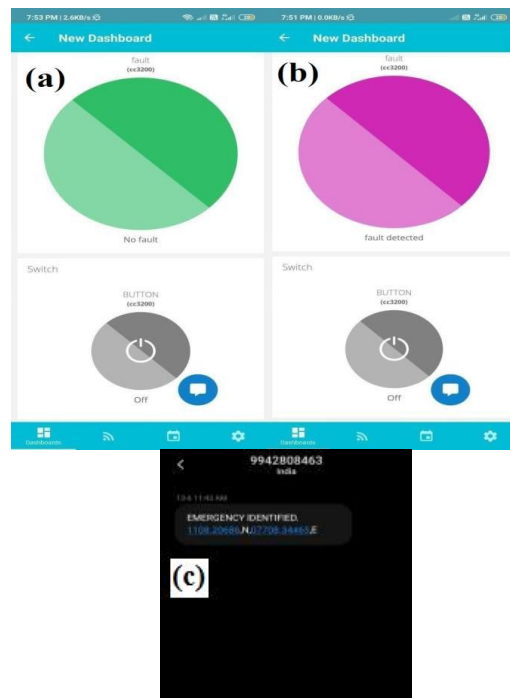
Fig. 3 (a) No fault (b) Fault detected screen of the UBIDOTS mobile application (c) SMS notification
