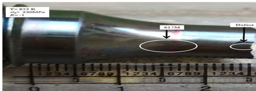
Fig.4.13: Failure location of DDMW HCF tested sample at 853 K, \sigma_a = 230 MPa, R = -1 .
