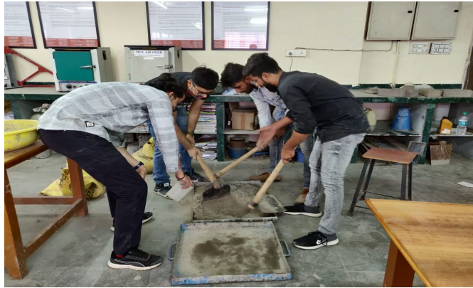
Fig. 2 Group members casting concrete blocks
