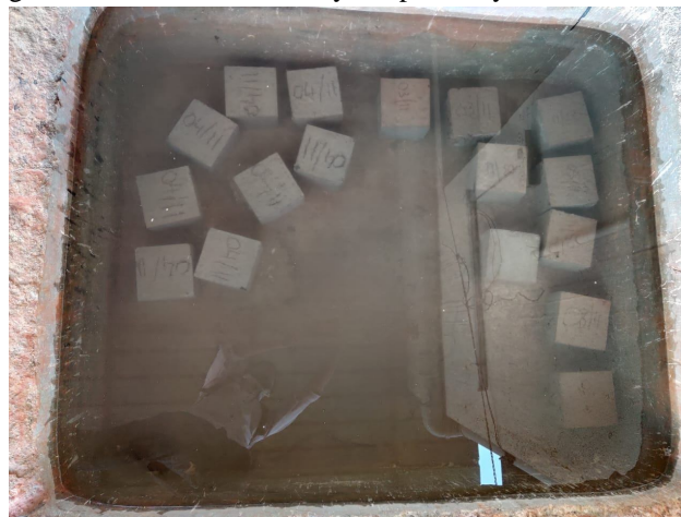
Fig. 3 Concrete blocks placed for curing in curing tank
