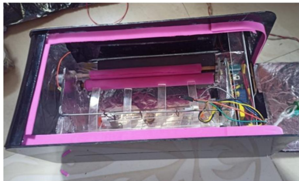
Fig. 2 Design Of Currency Sanitizer Using UV-C Light
