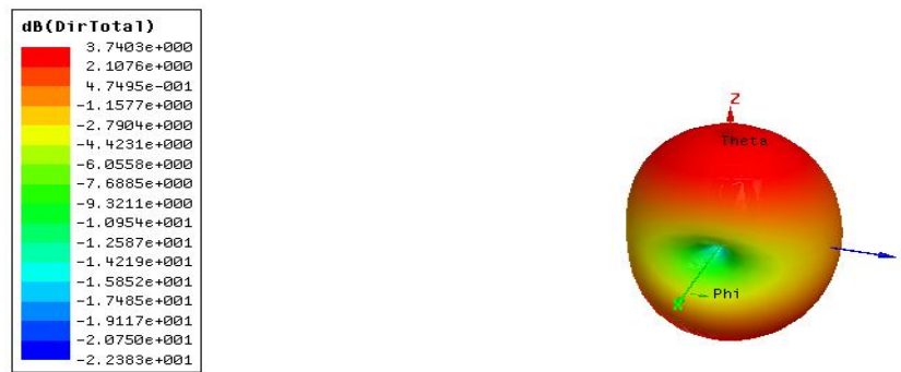
Figure 3.6: 3-D polar plots for mirostrip patch antenna at 3 GHz
