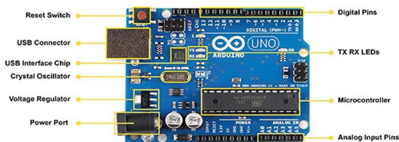
Figure 3.5 Pin diagram of Arduino-Uno AtMega328
