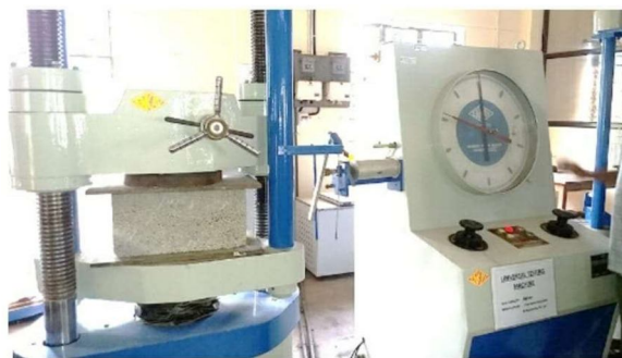
Fig 2. Testing of Solid Concrete Block
