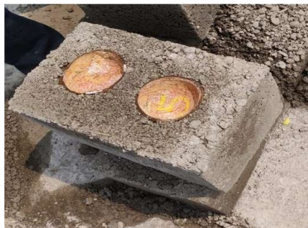
Fig.1 : Solid Concrete Block casted with Coconut Shell
