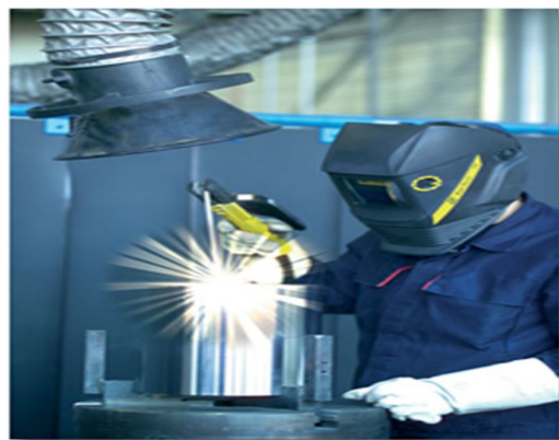
Fig No 15: performing arc welding
