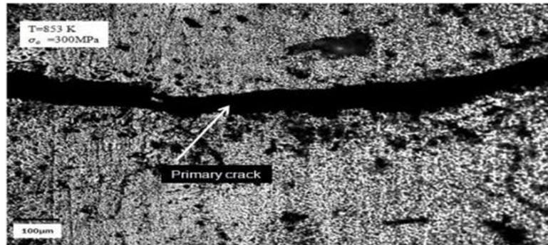
Fig.4.8: Replica image indicating the surface damage of 10wt%Cr Steel at 853 K, \sigma_a = 300 MPa, R = -1 .
