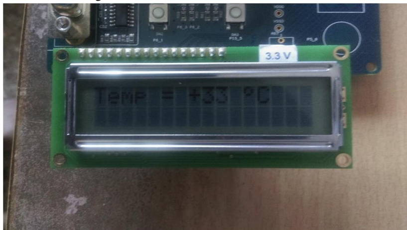
Fig 9 Temperature Sensed by PSOC displayed on LCD
