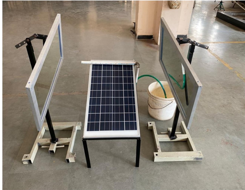
Figure 3.1. Working set up with cooling and reflector arrangement
