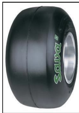
Fig. 3. Typical go-kart slick tire.
